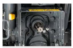
**POWER TAKE-OFF** PTO shaft with operating ranges 540/540E and standard.
