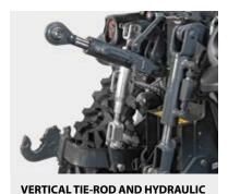
**THIRD-POINT**Optimizes the positioning and inclination of the equipment.
