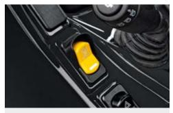
**CONTROL TO KEEP PTO RUNNING**This control keeps the PTO engaged and running even when the operator leaves the seat.
