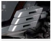
**FRONT BALLAST**Perfectly integrated into the bodywork of the tractor; it does not alter the wheelbase or dimensions of the tractor.
