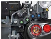
Electro-proportional hydraulic system controlled by joystick with double driver safety system and integrated control unit with user-adjustable settings - 12 rear quick couplings. External lifting control.
