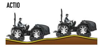
Thanks to the 45° offset of the front and rear axle final drives, the Mach 4 combines a long wheelbase with a reduced engine overhang: features which grant perfect stability in all operations, ensuring maximum safety and comfort at all times.
