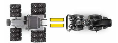
The four alternate-grip rubber tracks (w: 13,78 in), similar to "ground profile" tyres, assure constant adherence during all manoeuvres, even on slippery ground.
