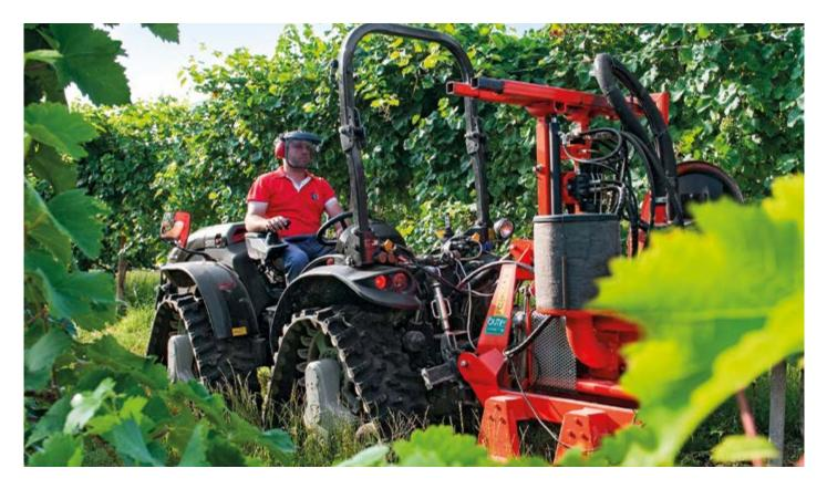
The lighting system, incorporated in the mudguards, features parabolic reflector units for a longer view of the track ahead, the implement and the surrounding area. Servicing is quick and easy thanks to the fully-opening bonnet and easily removable engine compartment side panels and battery cover.
