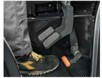
**STEERING BRAKES**Steering brakes have been introduced to further reduce the turning radius.
