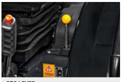
**PTO LEVER**This command selects the PTO shaft in independent or synchronised mode.
