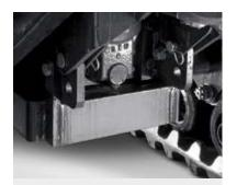
**BALANCING BALLAST**Supplementary ballast for optimising vehicle balance.
